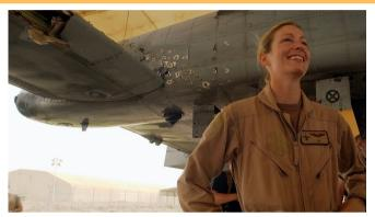
A great example of redundant systems is the A-10 Warthog, a plane used by the US Air Force for almost 50 years. The aircraft's purpose was close combat support and needed to work even when taking enemy fire. Its entire design was built on redundant systems. If one system failed, another kicked in.
